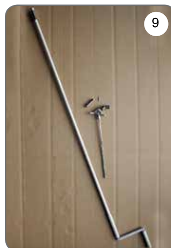
Handle, Cardan joint 45° or 90° with hook for Cardan joint [9].
